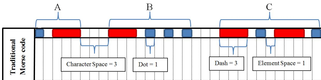
**Figure 1.3:** Morse code timing scheme. Morse code elements are distinguished in terms of the amount of time units a stimulus is active or inactive. Dots and dashes are represented with active stimulus contributing 1 and 3 time units respectively. Element gaps, letter gaps and word gaps are represented with inactive stimulus at 1, 3 and 7 time units respectively.
