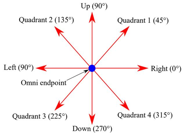
Figure 4.4: All force perturbation conditions are shown in a 2D plane acting on the Omni endpoint. There were nine total force conditions with the one condition not shown being the no force, baseline condition. The naming conventions seen in this figure will be used consistently throughout this thesis.
