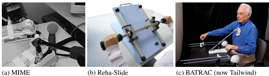
Fig. 5 Several of the devices that have been used for bimanual rehabilitation. The general idea of bimanual rehabilitation is that an individual assists his own paretic arm with his sound arm through an external physical coupling. Subfigure (a) reproduced from [48] under the Creative Commons Attribution License. Subfigures (b) and (c) reproduced with permission.
