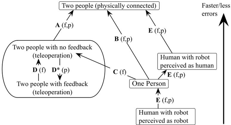
**Fig. 7.1** Summary of several experiments that compare the speed and error rate of several algorithms for mediating human-robot-human interactions. Each of these used a second order inertial system, except for D\*, which used a zero-order system. An ‘f’ indicates that the other member’s force was displayed while a ‘p’ indicates position was displayed (A—Summers et al. [16] and Field et al. [17]; B—Reed et al. [18, 19]; C—Glynn et al. [20]; D—Glynn et al. [21]; E—Reed et al. [22, 23])
