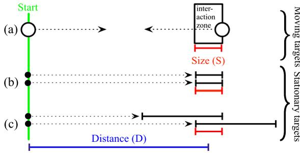
**Fig. 7.2** The variations of Fitts' Law for two people. (a) The target is the other person's hand, so the target is moving toward as each member of the team attempt to reach the target. This type of experiment was performed in [7, 31]. (b) The target is stationary and the two members work together to reach the same target [32]. (c) The two individuals have different, but overlapping, targets, so they must physically work together to reach the target [32]
