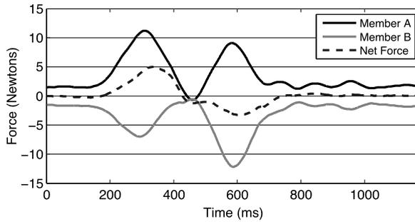
**Fig. 7.4** The dyad specializes, which is where each member only pushes in one direction. Each member contributes to certain aspects of the task: member A accelerates while member B decelerates. The forces sum to a force profile similar to an individual performing the task. Figure used with permission from [23] (© 2007 IEEE)
