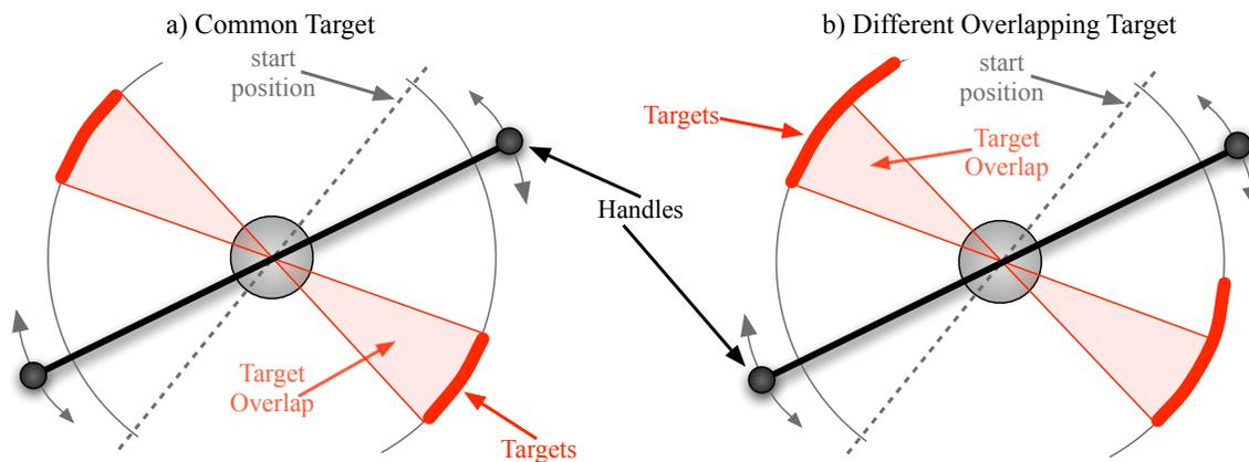
Figure 4.2. Comparison of the two parts of the Fitts' law experiment. a) The common target experiment (shown on the left) requires no negotiation between the subjects since their targets are exactly the same. b) The different overlapping target experiment requires the subjects to compromise by moving into a subset of their target that also satisfies their partner's target. The subjects only see their own target, not their partner's.
