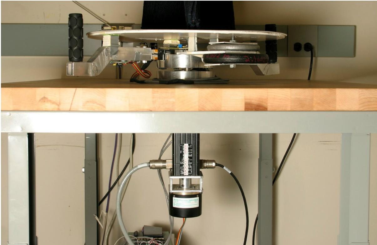
Figure 2.2. View of the device from the side, both above and below the table. The direct drive motor is attached under the table and out of the view of the users.
