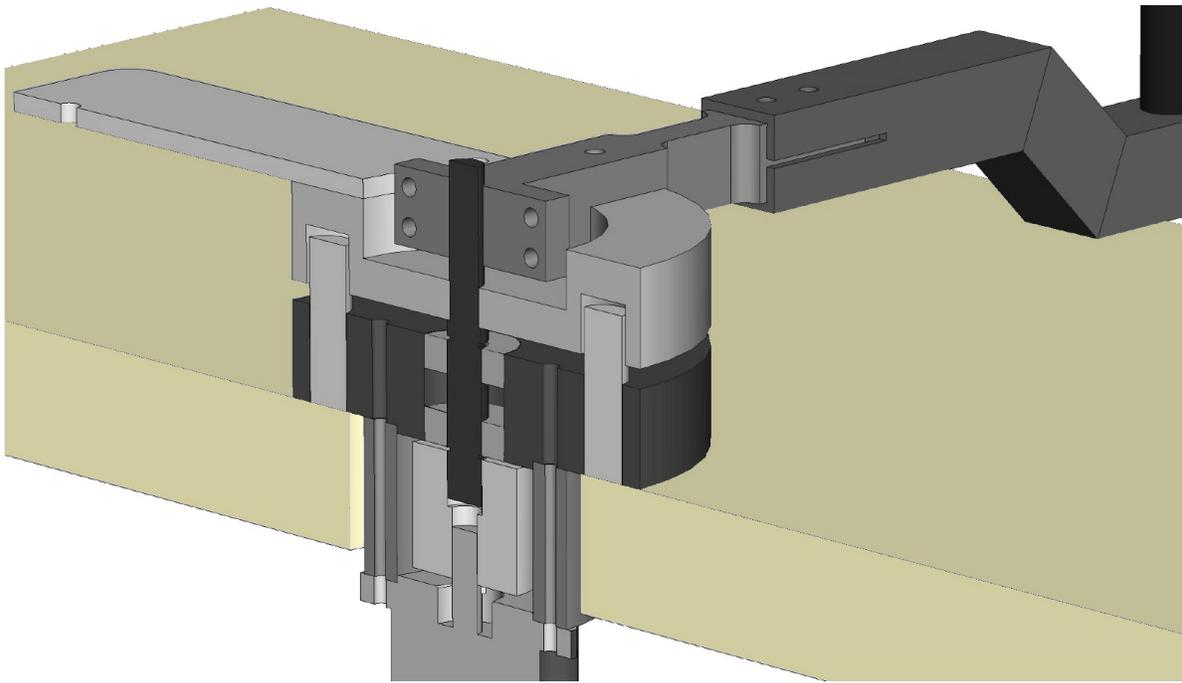
Figure 2.3. Internal view of the center of the device. This view shows the internal connections between the motor, handles, and table. The bearings support all forces and moments from the handles.
