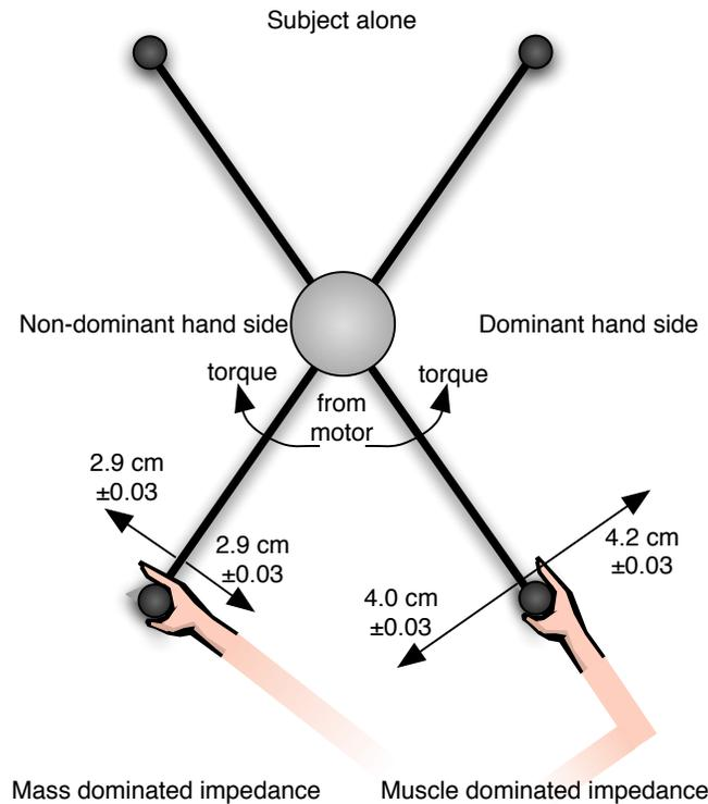
Figure 5.4. Configuration of the individual trials. The motor applies a torque that simulates the dyadic-contraction force. The motor also applies a perturbation force that results in a displacement (shown with the confidence intervals). The displacement difference between the dominant and non-dominant sides is largely due to the arm configuration. The displacement difference on the dominant side is largely due to different muscle impedance in each direction.
