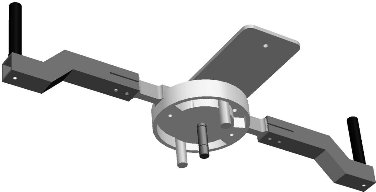
Figure 2.4. View of the crank handle bars from underneath. This reveals the groove in the bottom of the top plate that prevents the crank from spinning in a complete circle. The removable stopper shafts are mounted to the bottom plate (not shown) to limit the range of motion.
