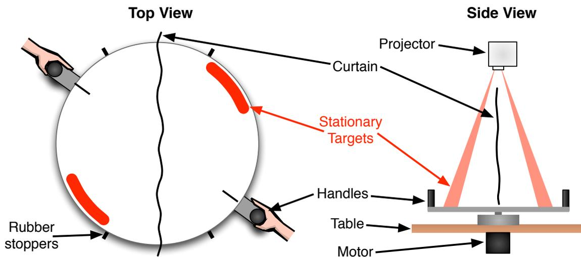
Figure 3.2. Diagram showing the setup of the device used for experiments.
