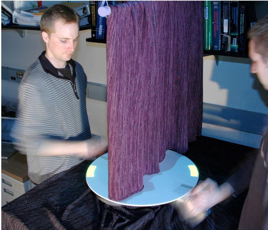
Figure 3.1. Two-handed crank setup used for experiments. A projector displays the targets from above. A curtain hangs between the two subjects to prevent non-physical communication.
