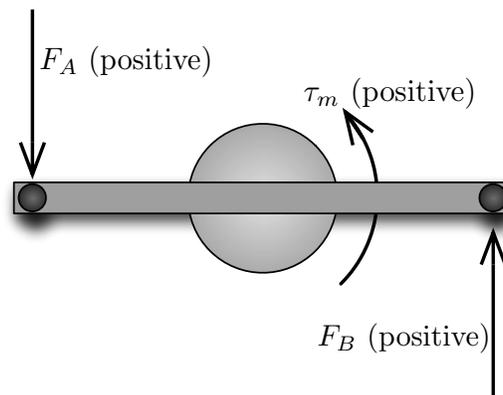
Figure 2.5. Definition of forces and torques on the crank.  $\tau_m$  is the motor torque calibrated to match an equivalent force at the handle.  $F_A$  is the force at one of the handles and  $F_B$  is the force at the other handle.
