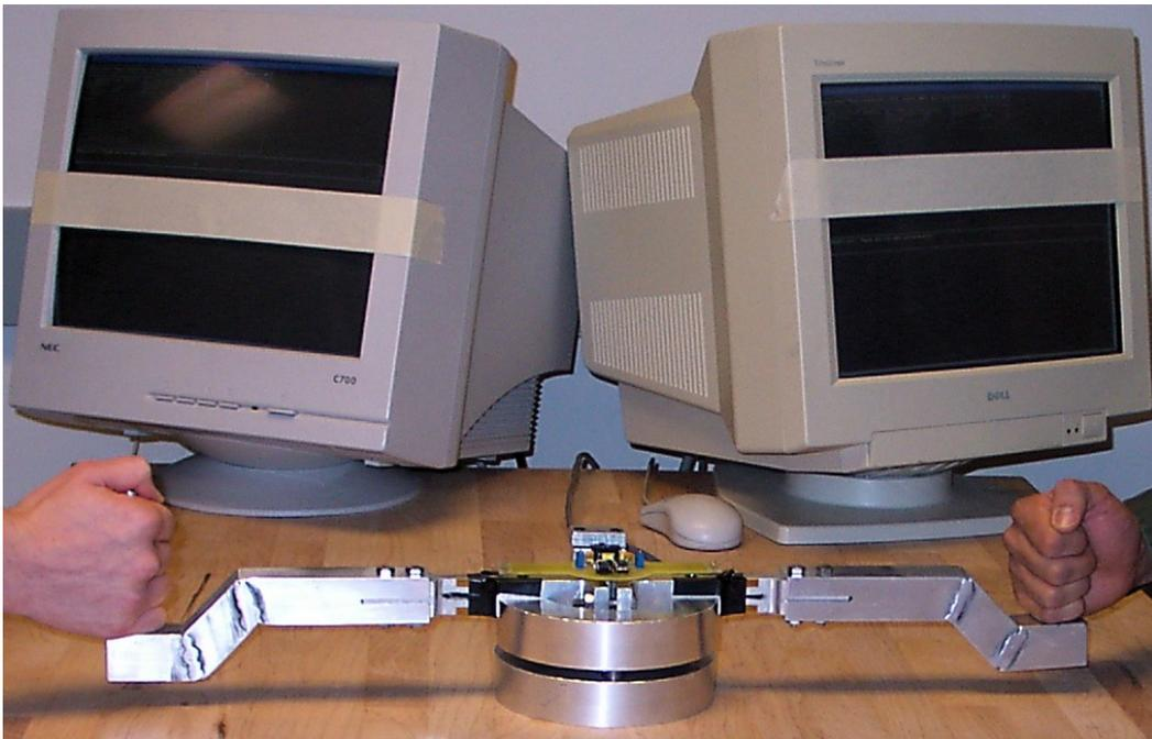
Figure 4.1. Initial device setup without curtain and without top plate. The targets are displayed on the computer screen along with the current position of the crank.
