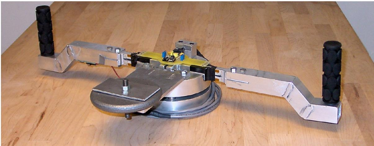
Figure 2.1. Top view of the mechanical device used for experiments. Two users grab the handles, one on either side. This device can measure the force applied to each handle, the angular acceleration of the crank, and the angular position of the crank.
