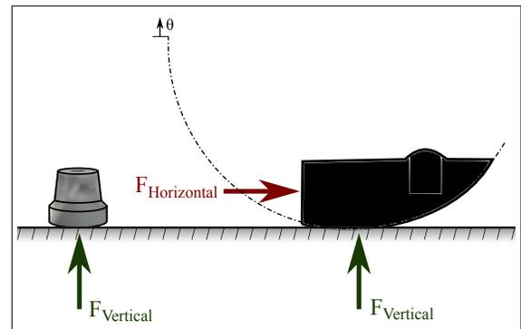
Fig. 3. Ground Reaction Forces to Kinetic Crutch Tip and Standard Tip
