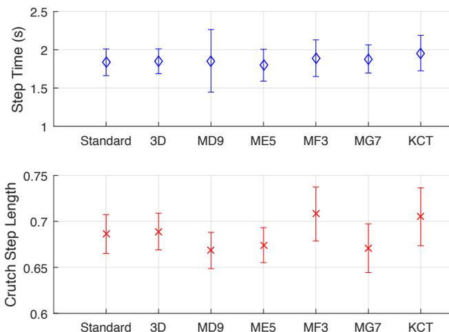
Fig. 8. Crutch Step Time and Length for Different Crutch Tips
