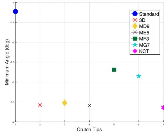
Fig. 6. Maximum Backward Rotation Angle for Different Crutch Tip
