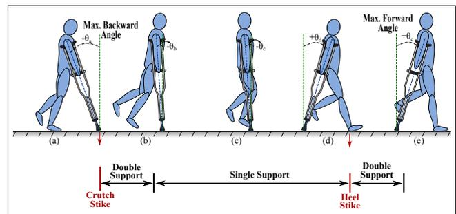
Fig. 7. Swing through crutch gait cycle
