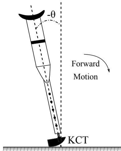
Fig. 2. Crutch Forward Motion with Backward Angle
