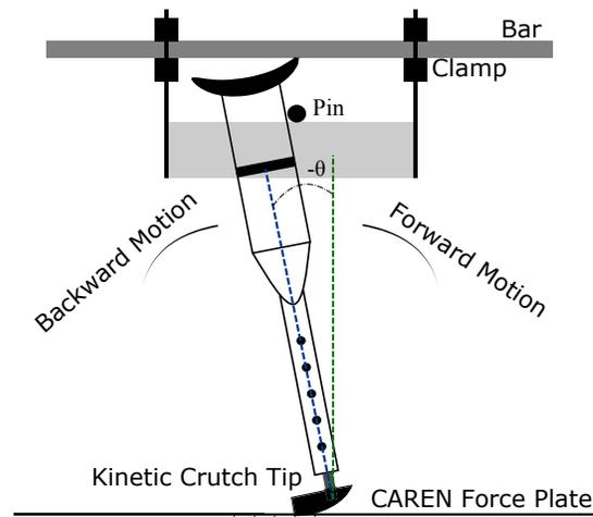
Fig. 4. A schematic of the setup for Crutch Free Fall Experiment
