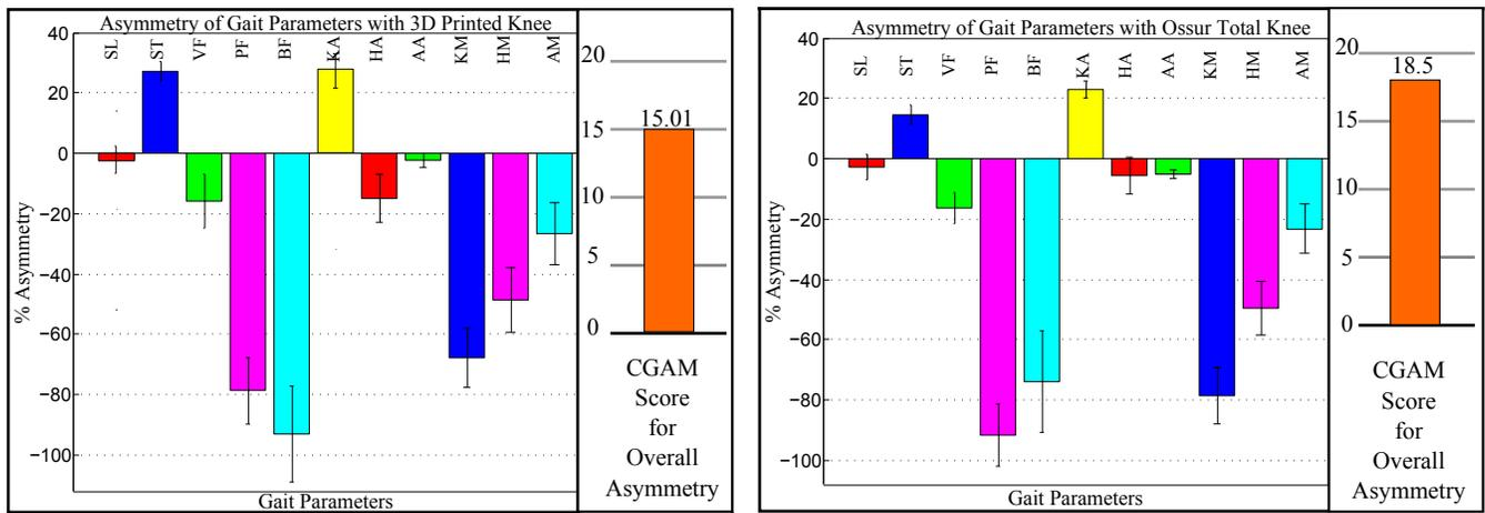
Fig. 5. CGAM Scores; [Legend: SL–Step Length, ST–Step Time, VF–Vertical Force, PF–Push Off Force, BF–Braking Force, KA–Knee Angle, HA–Hip Angle, AA–Ankle Angle, KM–Knee Moment, HM–Hip Moment, AM–Ankle Moment]
