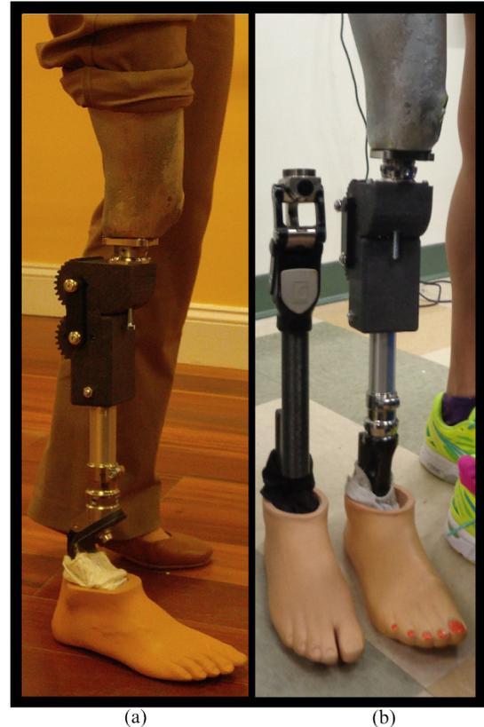
Fig. 2. Amputee wearing the 3D printed knee. (a) Side view and (b) Ossur 2000 next to the 3D printed knee.
