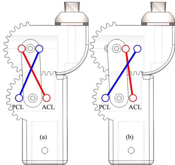
Fig. 1. Spring Configuration. (a) The configuration used in the experiments. (b) Configuration for faster extension.
