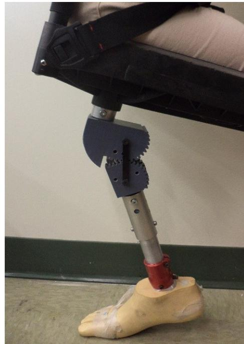
Figure 9. 3D Printed Prosthetic Knee Fitted on the Simulator
