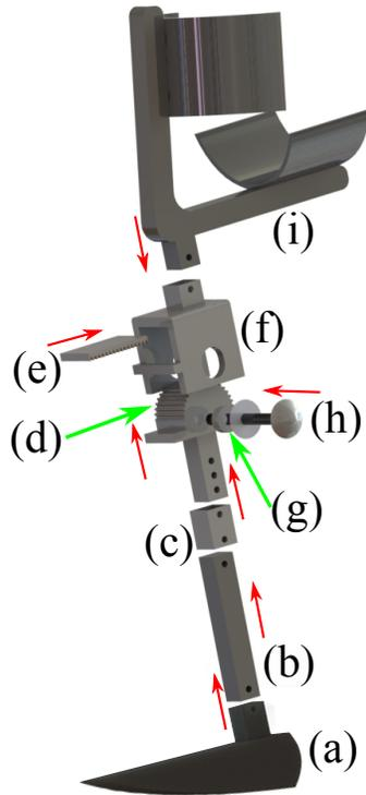
**FIGURE 2.** Exploded view of the prosthetic simulator: Red arrows indicate assembly direction and green arrows indicate specific components: (a) prosthetic foot based on roll-over shape, (b) extender component, (c) coupling, (d) shank with spur gear, (e) femoral spur gear rack, (f) femoral housing, (g) bearing, (h) shaft, and (i) knee brace
