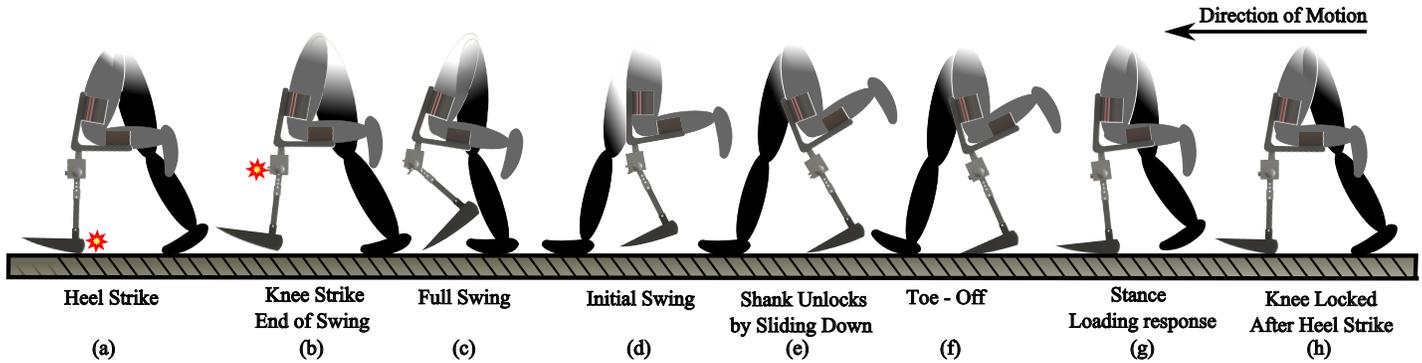
FIGURE 4. Example of walking with the prosthetic simulator.
