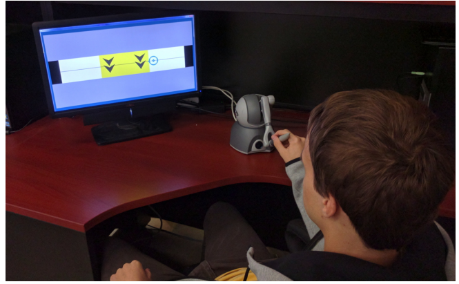
Fig. 1: The experimental setup with desktop computer and Geomagic Touch is shown here for the right hand configuration.
