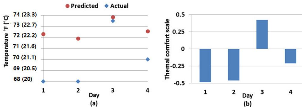
**Figure 3** The summer classroom temperatures. (a) The actual temperature of the summer class versus the average predicted temperature from subjects. (b) The average thermal comfort level of subjects for four days during summer class.
