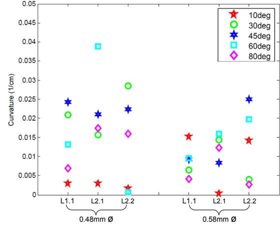
Fig. 6: Effects of bevel-tip angle ( $\alpha$ ) on shaft curvature for two different shaft diameters and three different insertions in two livers (one insertion into Liver 1 and two insertions into Liver 2).
