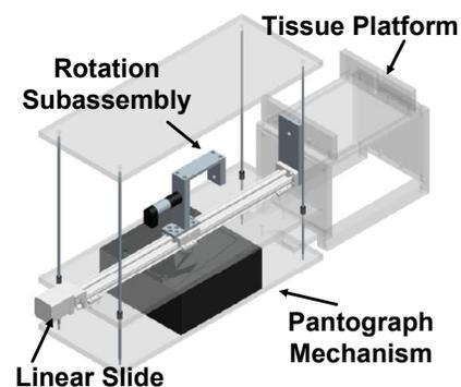
Fig. 1: Model of the portable needle steering device.
