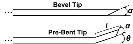
Fig. 4: Bevel-tip needles have a single angled tip defined by the variable  $\alpha$ . Pre-bent needles are characterized with a bend angle,  $\theta$ , and bend length,  $l$ . Pre-bent needles may also have bevel angles.
