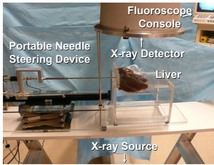
Fig. 2: Image of experimental setup, including the portable needle steering device, the fluoroscope, and the liver.
