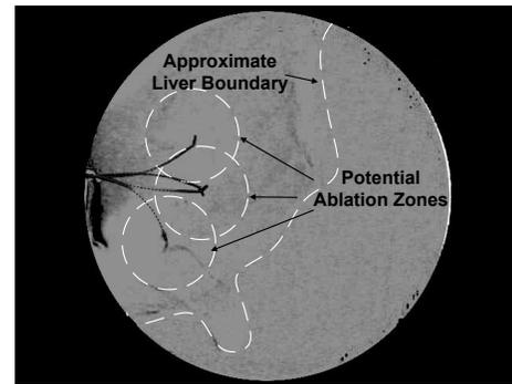
Fig. 8: Simulated ablation was performed in *ex vivo* liver as an example of a needle steering application. The steered needle was partially inserted and retracted several times with different tip orientations to demonstrate coverage of a region of interest.
