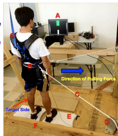
Figure 1. A prototype of robot-assisted balance training device. A: Monitor, B: Waist belt, C: Pulling cable, D: Pulley, E: Wii boards, F: Frame, and G: Safety harness
