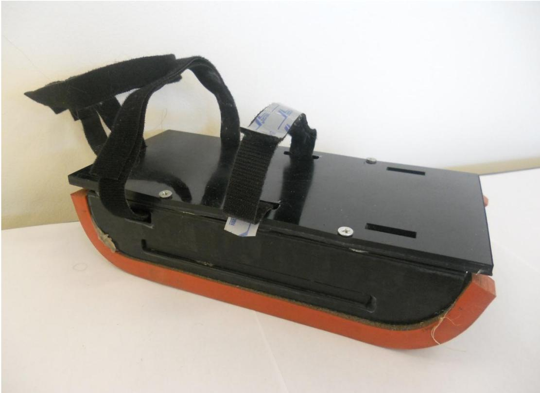
Figure B.1: Photo of shoe worn during the walking experiment. Worn on the left leg, it made the leg 2" taller and 4lb. heavier.
