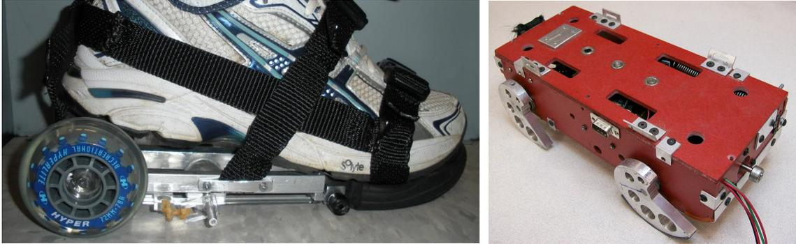
Figure 2.5: GEMS Shoe designs. The left shoe was developed by de Groot et. al [5] in 2009. This completely passive shoe uses a rack and pinion to convert the user's energy into a backwards motion. While the right shoe is also completely passive, it uses a magnetic particle brake to generate a more controlled motion.
