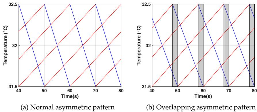
Fig. 2: Comparison of (a) normal and (b) overlapping constant cooling asymmetric thermal pattern. Each line corresponds to one actuator. Red lines are slowly heating and blue lines are rapidly cooling.
