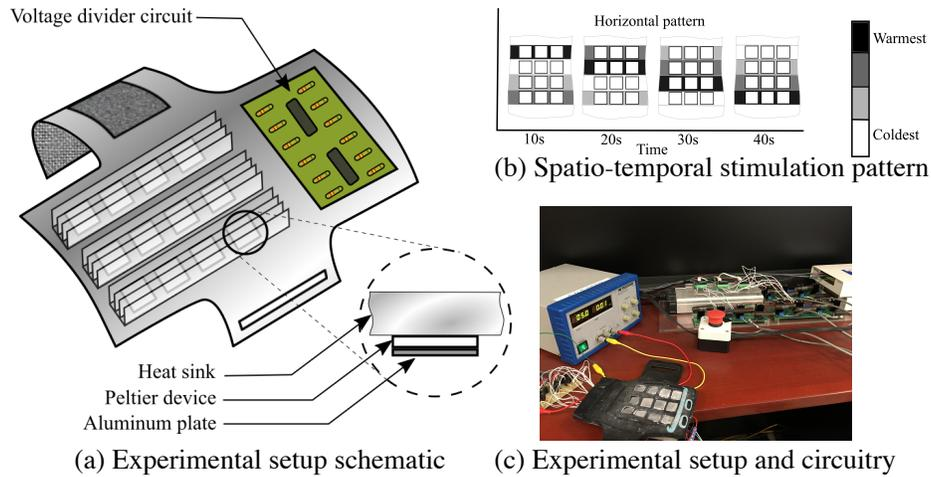
Fig. 3: Experimental setup schematic and stimulation pattern.
