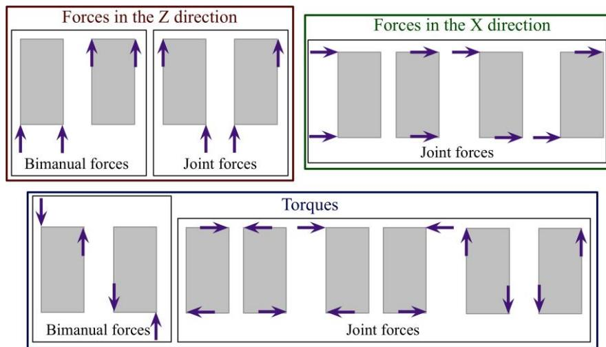
Figure 3. An example of the 16 redundant combinations that four forces from two people can create. Higher numbers of input forces leads to many more redundant combinations. These forces can be divided into bimanual forces/torques, which are those that arise from only one person, and joint forces/torques, which are those that arise from the interaction of the two individuals.
