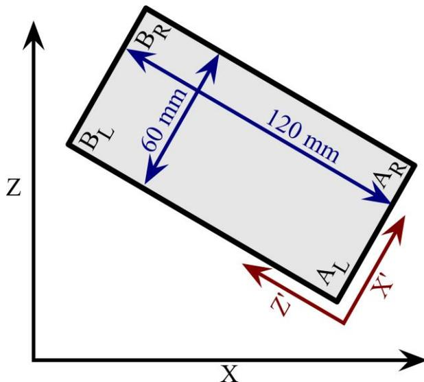
Figure 4. Two reference frames are used to analyze the planar interaction forces. One is the world frame, which is the view of the computer monitor and of the Omni. The second is the boxframe, which is the moving frame attached to the box, indicated by  $X'$  and  $Z'$ .  $A_L$ ,  $A_R$ ,  $B_L$ , and  $B_R$  correspond to the left and right hands of members A and B, respectively.
