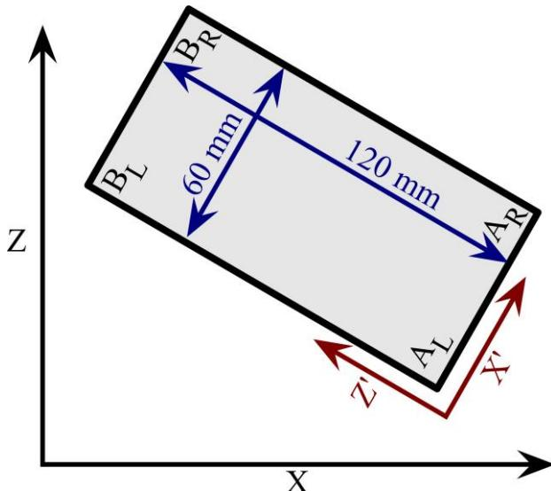
Figure 4. Two reference frames are used to analyze the planar interaction forces. One is the world frame, which is the view of the computer monitor and of the Omnis. The second is the boxframe, which is the moving frame attached to the box, indicated by  $X'$  and  $Z'$ .  $A_L$ ,  $A_R$ ,  $B_L$ , and  $B_R$  correspond to the left and right hands of members A and B, respectively.
