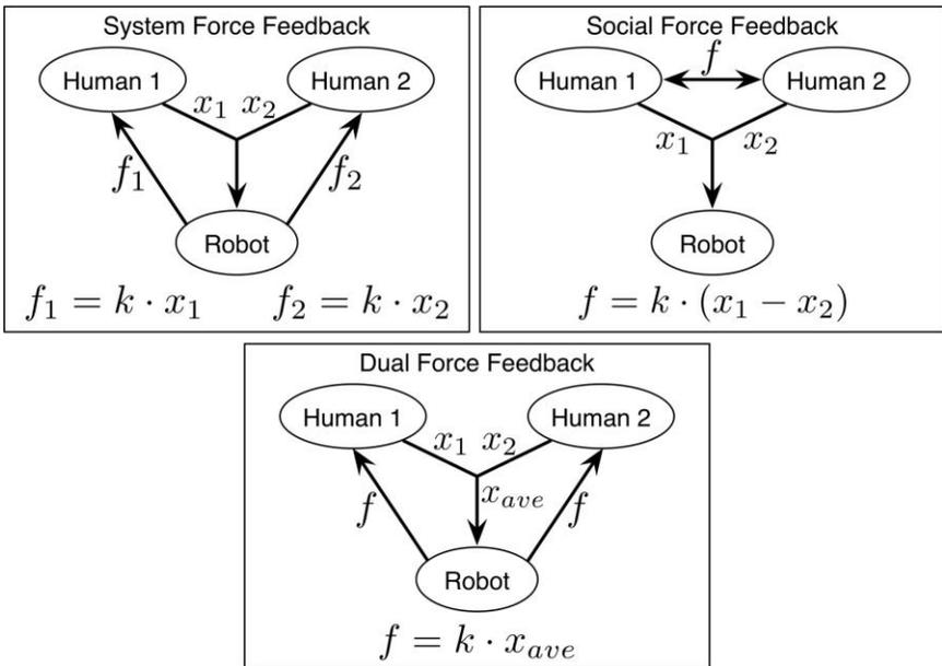
Figure 7. The three force feedback modes used in this cooperative interaction experiment. Each mode controls the slave to be the average of the two master robots. System Force Feedback is based on the individual position of each master. Social Force Feedback is based on the difference of the two master positions. Dual Force Feedback provides the same feedback to each user based on the average position of the two masters.
