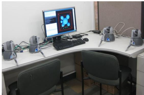
Figure 1. The complete experimental setup during the experiments. In this photo, the practice simulation has just begun, and all four haptic devices are activated and are seen hovering above the table as they are in fact resting on the floor of the virtual environment.
