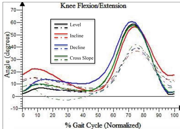
**Fig. 2** Average knee kinematics at various elevations: level (black), uphill (red), downhill (blue), and cross slope (green) walking in non-amputees (solid) and bilateral transtibial amputee (dashed)
