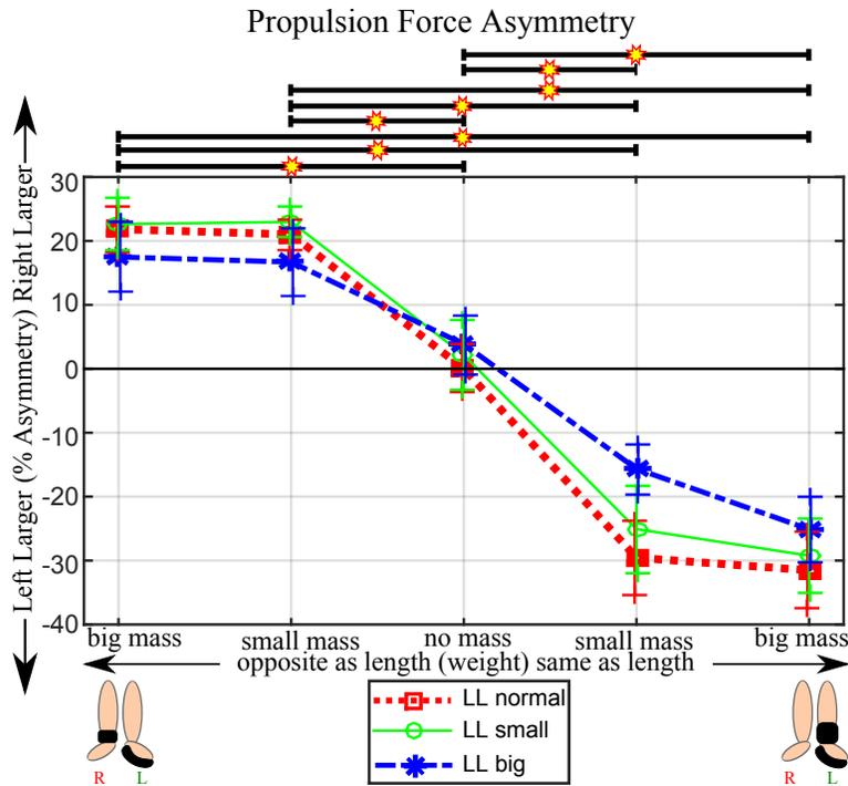
Figure 4.7: Peak Push off Force for All the Conditions. (Bars Show Standard Error)
