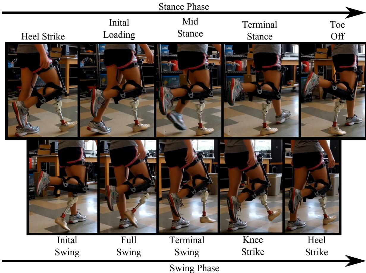
Figure 5.3: Able Body Subject Walking on Prosthetic Simulator with Gait Phases.
