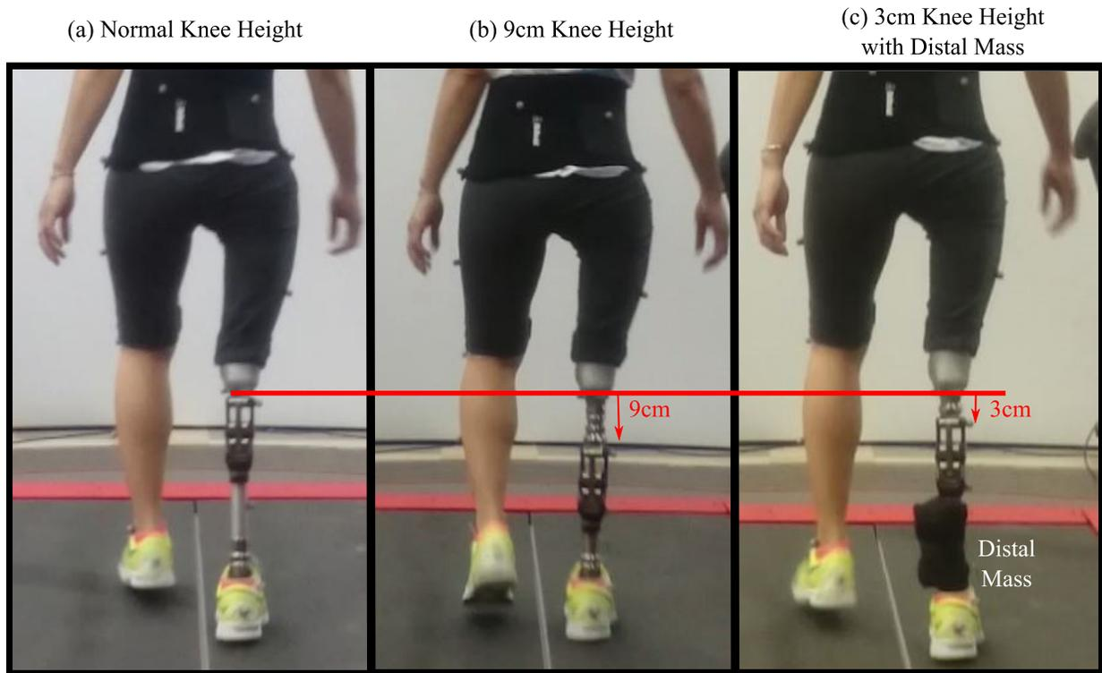
Figure 5.5: Amputee with Different Knee Heights and Distal Mass.
