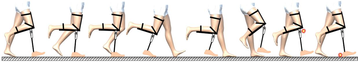
Figure 5.2: Able Body Subject Walking on Prosthetic Simulator.
