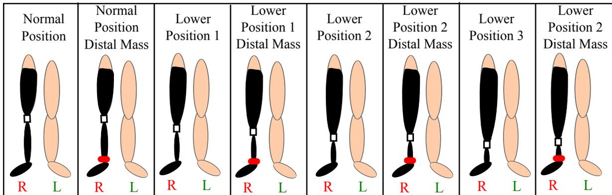
Figure 5.6: Different Perturbations of Knee Heights with a Combination of Distal Mass.
