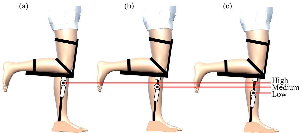
Figure 5.1: Prosthetic Simulator with Different Knee Heights.
