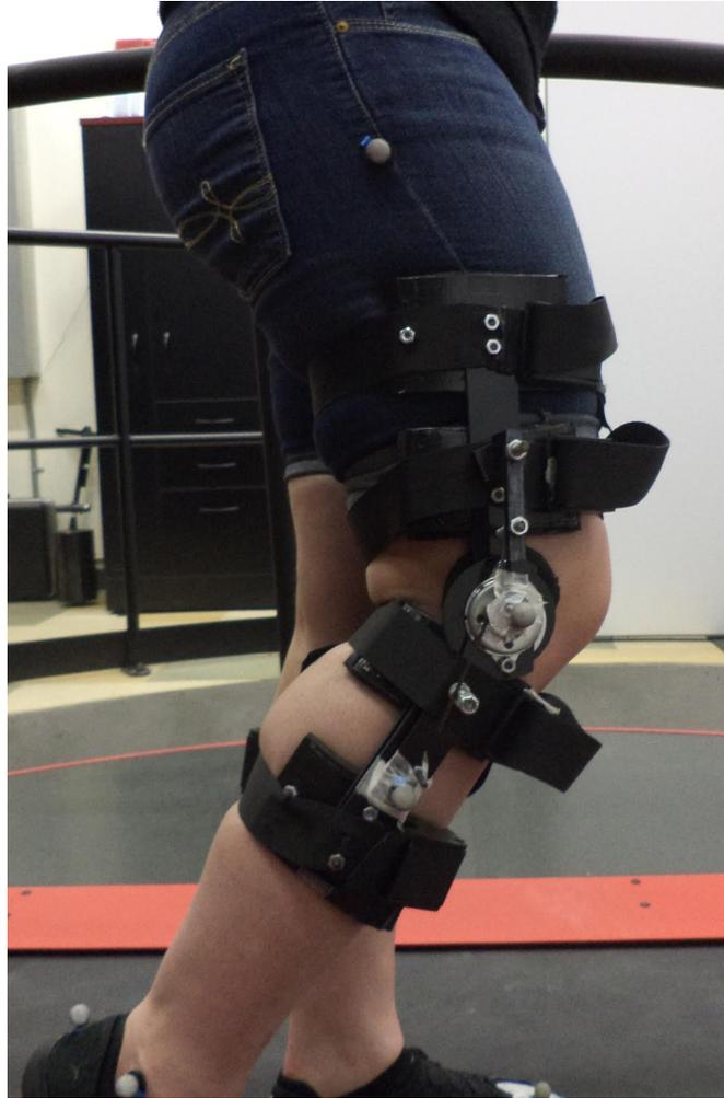
Figure 4.1: Stroke Simulator on a Subject.
