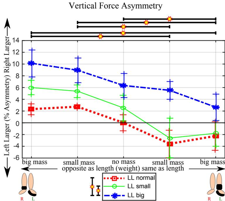
Figure 4.6: Peak Vertical Force for All the Conditions. (Bars Show Standard Error)
