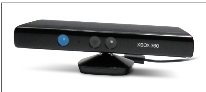
Fig. 2: Front view of an XBOX Kinect and its three sensors. From left to right, the IR projector, the RGB camera, and the monochrome camera (used for depth imaging) [1][2]
