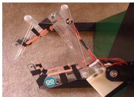
**Figure 4: Full assembly including FSR sensors and silicone tabs**
