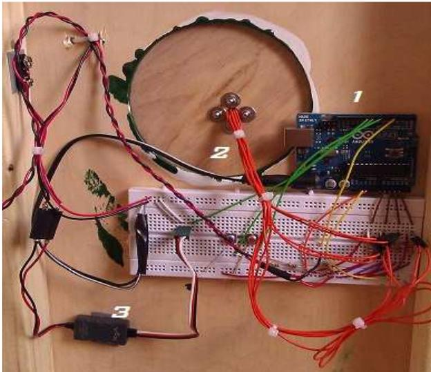
**Figure 5: Control System: (1) Micro-controller board, (2) FSR wiring, (3) Motor controller**
