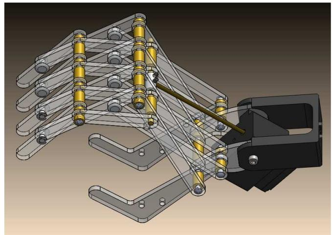
**Figure 1: 6-bar linkage gripping mechanism actuated via power-screw**
