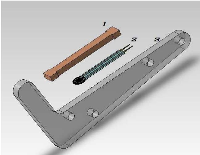
**Figure 2: (1) Silicone tab, (2) FSR, (3) Linkage**
