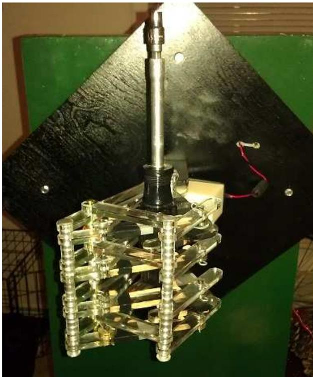
**Figure 7: Mechanism gripping a small cylindrical object**
