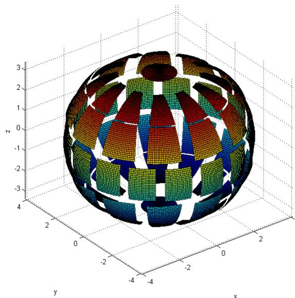
Fig. 3. The angular regions able to be communicated by this particular design.
