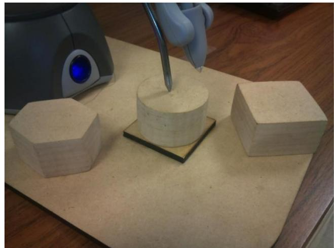
Figure 3: Testing Apparatus. Simple shapes and extended end effector.
