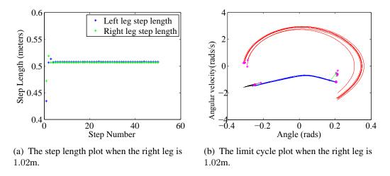
Figure 4.3: The symmetric solution when the right leg is 1.02m. This happens by adding a mass on the left leg shank and thigh with a magnitude of 0.0025kg and 0.025kg respectively. The mass on the thigh is located on the knee (b2L = 0.25m) and the shank mass is 0.1m above the center of the shank
