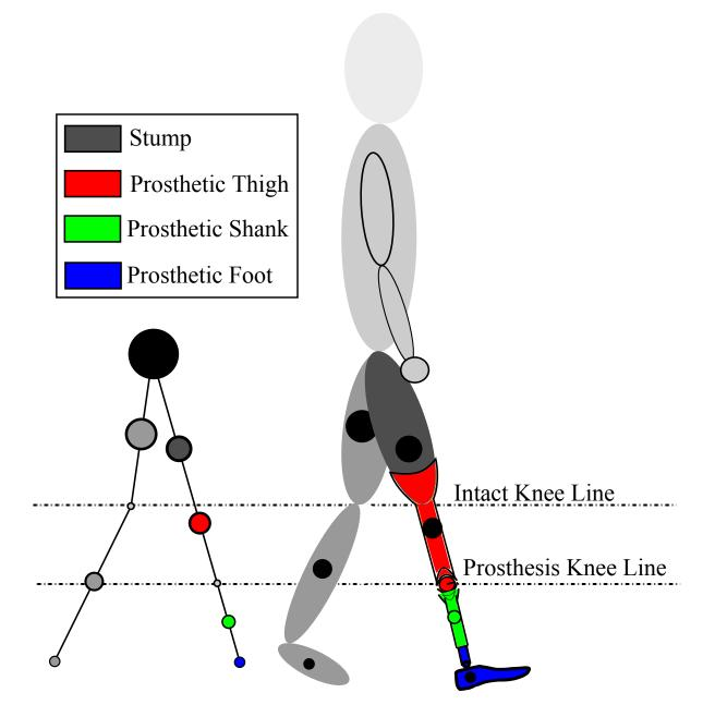
Figure 4.9: The prosthesis model. This shows the prosthesis model that was derived to better represent a transfemoral prosthetic leg.
