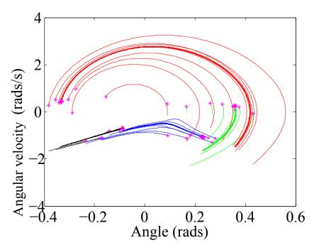
(b) Limit cycle plot for the prosthesis model when the total mass is heavier and the gait patten is symmetric.
