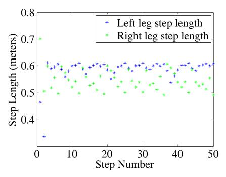
(a) Step length plot for the prosthesis model when the total mass is lighter and the gait patten is asymmetric.
