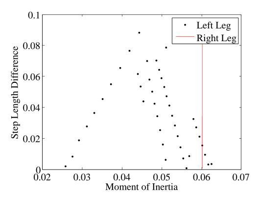
(a) Moment of inertia of the left leg when the right leg shank mass is spread out by 0.24m.
