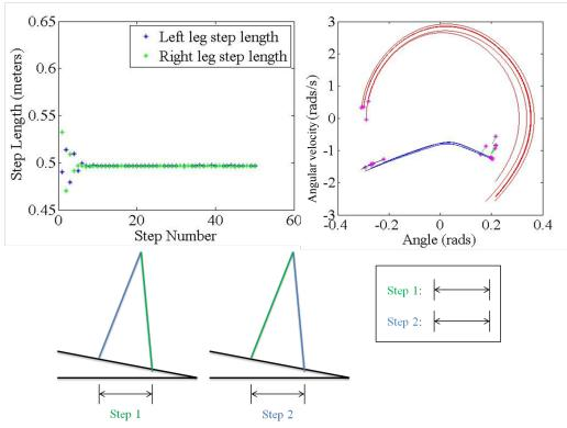
Figure 2.4: The symmetric step pattern.
