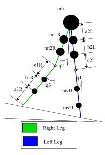
Figure 3.2: The nine mass three link model.
