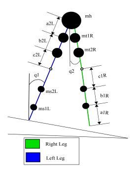
Figure 3.3: The nine mass two link model.
