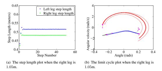
Figure 4.6: The symmetric solution when the right leg is 1.05m. The most symmetric solution happens when the left leg has a thigh mass equaling 0.025kg and is located at the center of the thigh and has a shank mass of 0.0025kg and is located 0.1m below the knee.
