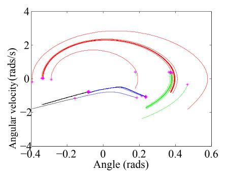
(b) Limit cycle plot for the prosthesis model when the total mass is lighter and the gait patten is asymmetric.
