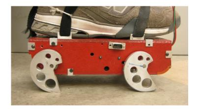
Figure 2.8: The gait enhancing mobile shoe (GEMS). [9]
