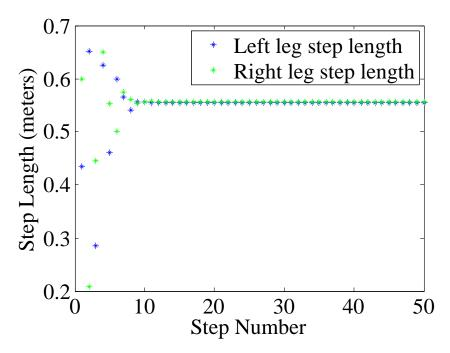
(a) Step length plot for the prosthesis model when the total mass is heavier and the gait patten is symmetric.
