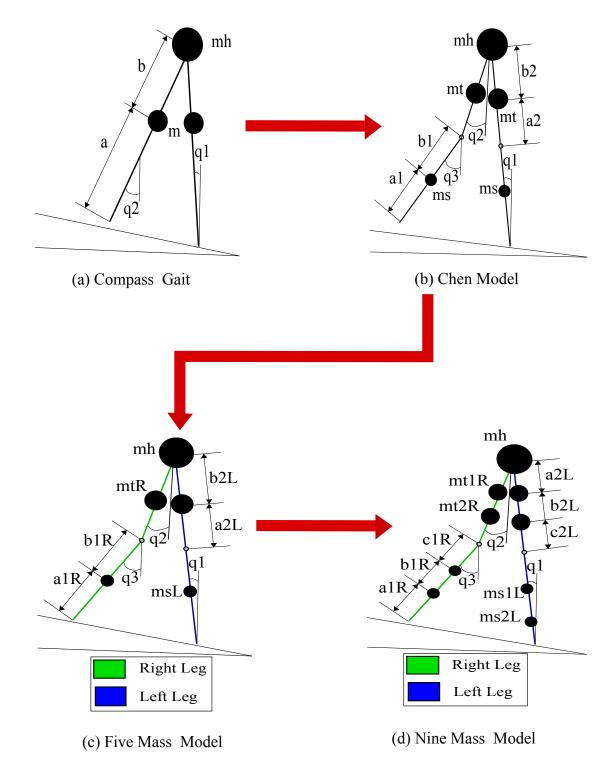
Figure 2.2: This shows evolution of the walker models. Starting with the compass gait [7], Chen's kneed model [1], the five mass model [11], and the nine mass model.
