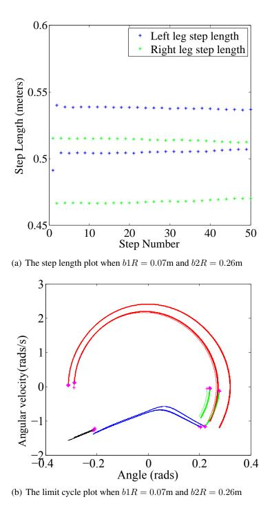
Figure 3.6: The masses on both the shank and thigh right leg are separated by 0.07m and 0.26m. This separation results in an asymmetry equaling 0.0300m.
