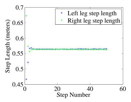
(a) Step length plot for the prosthesis model when the total mass is lighter and the gait patten is symmetric.
