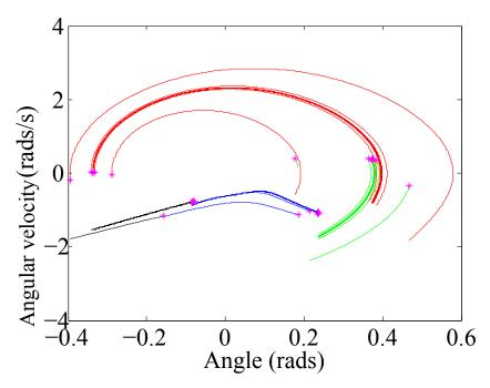
(b) Limit cycle plot for the prosthesis model when the total mass is lighter and the gait patten is symmetric.
