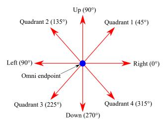
Figure 4.4: All force perturbation conditions are shown in a 2D plane acting on the Omni endpoint. There were nine total force conditions with the one condition not shown being the no force, baseline condition. The naming conventions seen in this figure will be used consistently throughout this thesis.
