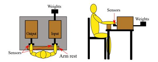
Figure 3.2: A schematic of the recreation device showing the force sensors, weights, and experimental setup.
