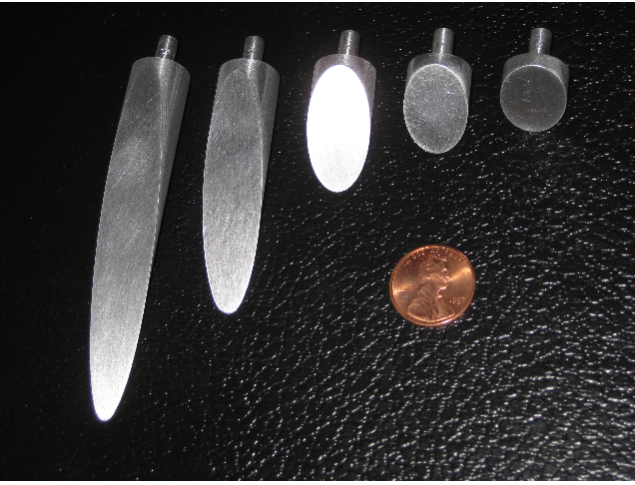
Fig. 4. Scaled needles of \text{\O}1.5 cm used to understand the interaction between the needle tip and medium. Needles of various bevel angles ( 10^\circ , 15^\circ , 30^\circ , 45^\circ , and 60^\circ ) were used in the study.
