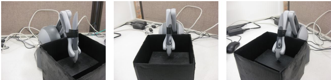
Figure 5. The materials analysis experiment in progress, as seen from the left, front, and right side. This is the second of two experiments which measures the ability of two human subjects to interact with a robot to perform an actual experiment and acquire data. All of the materials are painted black and are placed inside of a black box so that the subjects cannot easily determine the material's identity from sight alone.
