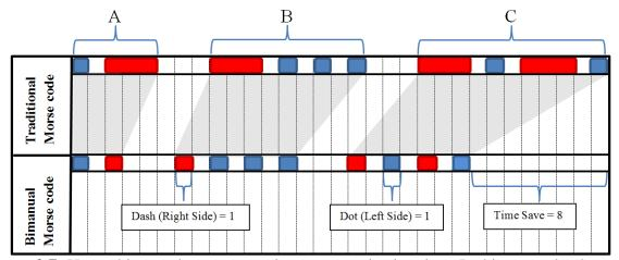
**Figure 2.7:** How a bimanual setup can reduce communication time. In this example, the string "ABC" is expressed 26% faster.
