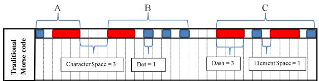
**Figure 1.3:** Morse code timing scheme. Morse code elements are distinguished in terms of the amount of time units a stimulus is active or inactive. Dots and dashes are represented with active stimulus contributing 1 and 3 time units respectively. Element gaps, letter gaps and word gaps are represented with inactive stimulus at 1, 3 and 7 time units respectively.
