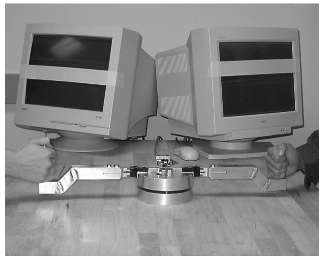
Figure 4. Experimental setup with two monitors and two-handed crank. The monitors display identical images, but the task for the other person is covered up, so that each subject sees only his or her own task.
