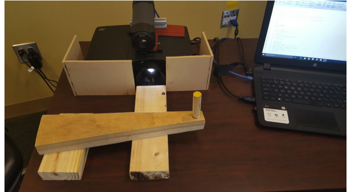
FIGURE 2. System set up. The figure shows the Optima projector with the FLIR thermal camera mounted on the top of the projector, along with the fixtures developed to block the exhaust coming from the projector and the fixture where the subjects will place their arm.
