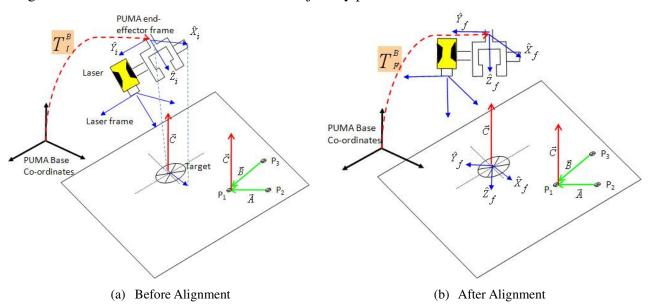
Figure 3. Concept - Laser based autonomous surface orientation by recording three surface points
