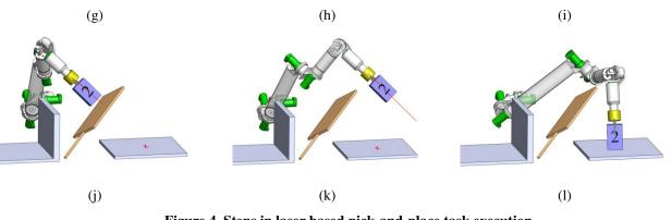
Figure 4. Steps in laser based pick-and-place task execution
