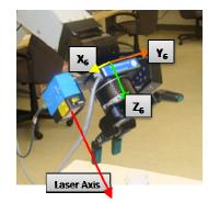
Figure 1. Laser sensor mounted on the end-effector
