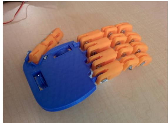
Figure 1. The 3D printed hand, force sensors have not been installed.
